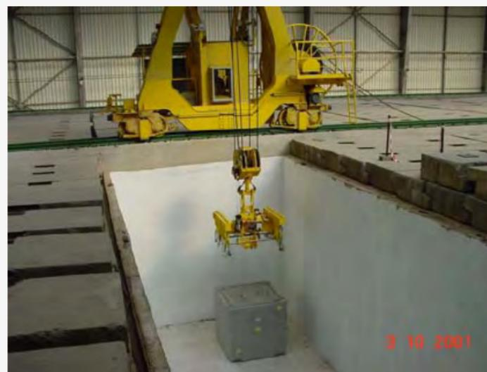
Picture 36: Fixed matrix being cemented to the Fibre Concrete Container.
