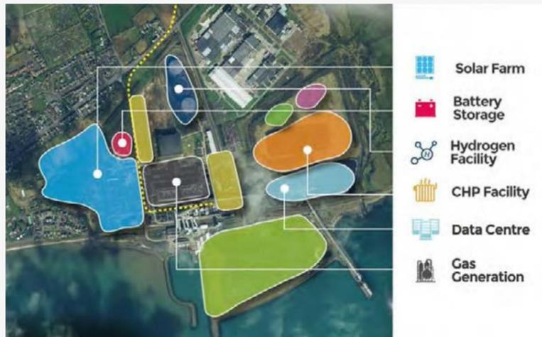
Picture 2: Conceptual layout of Kilroot Energy Park, representing the project's potential to contribute to the decarbonisation of the Northern Ireland power sector.
